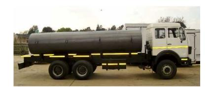
Mercedes Benz 26-28 Powerliner fitted with new 16000l water tank and full system. Ready to work. Also Included:
