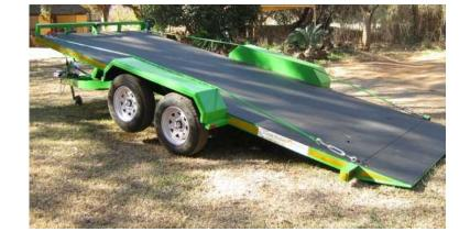
Loading area - Length 5m x 2m wide. Coupler - 3.5 ton. 2 x Brake Axle - 1.6 ton. Both axles are 3.2 ton. 4 x "14" Rim and Tyre. Jack - 2.5 ton to tilt the floor. Solid floor.
